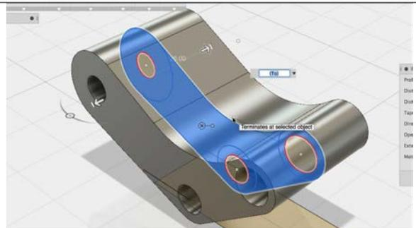
**Cut holes:** In this section you use the sketch profiles to cut holes in the body.
